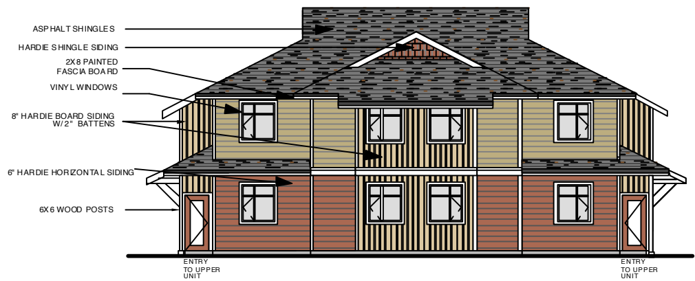
BLDG 5 STACKED TOWNHOUSE - FRONT ELEVATION SCALE 1/16"=1'-0"
