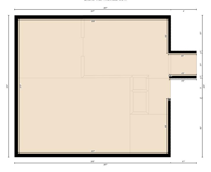
Measurement Diagram for: 1st Floor Exterior Wall Thickness: 6.5 in
