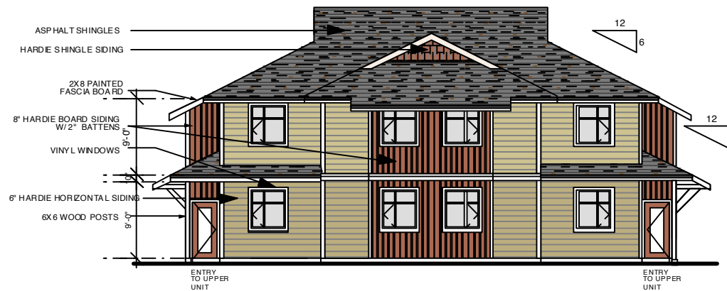
BLDG 4 STACKED TOWNHOUSE - FRONT ELEVATION SCALE 1/16"=1'-0"
