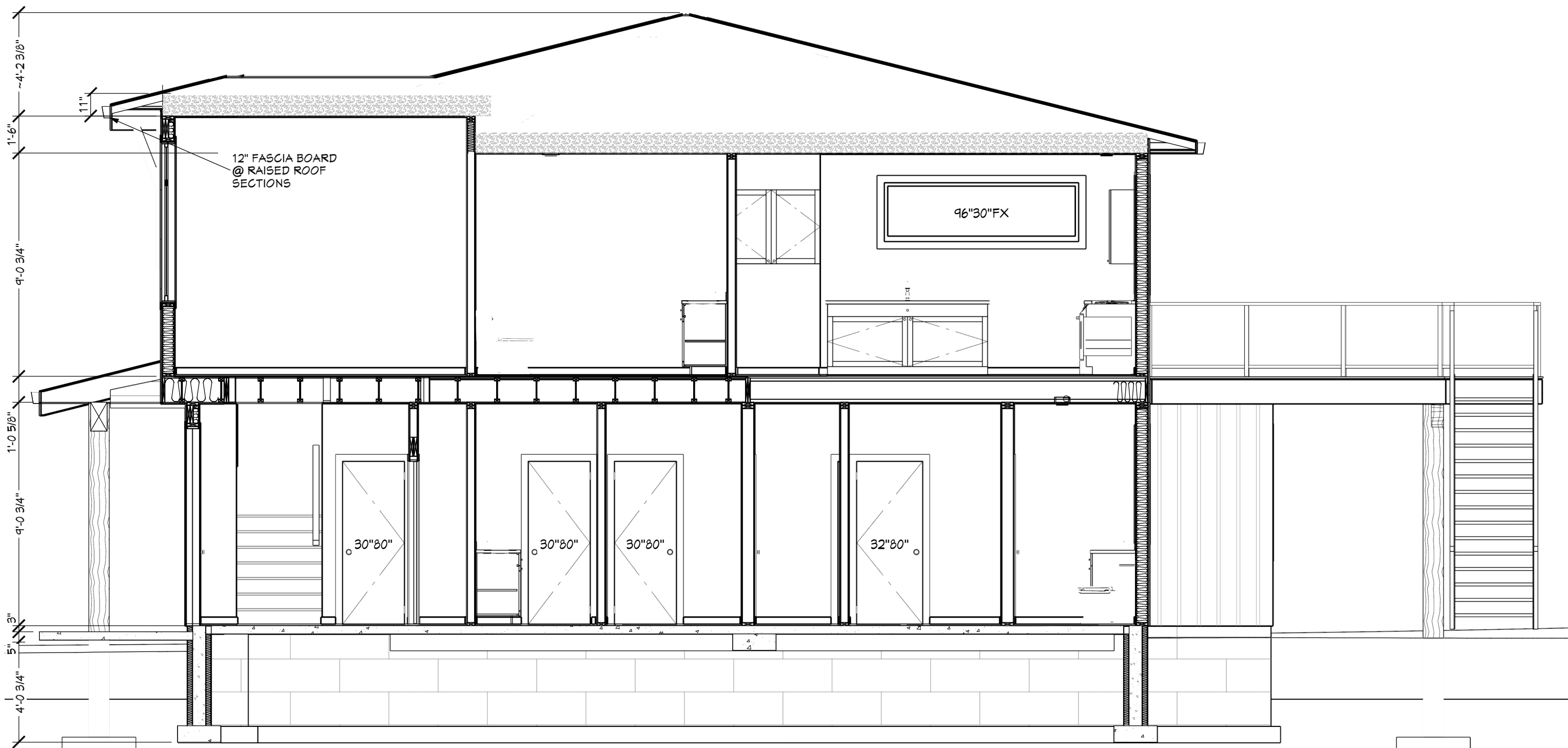
CROSS SECTION 1 SCALE: 1/4" = 1'-0"
